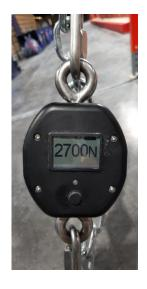
This easy to use tensiometer with measurement button and digital display **allows gymnasts to adapt the tension of the cables of the apparatus according to their needs** in competition as well as in training.
