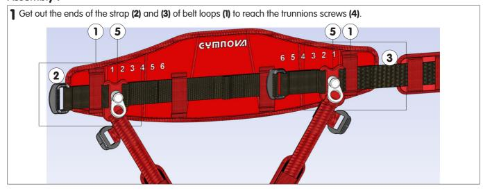
2 Remove the old system: dismount the screw (4) by keeping the support plate (5). Replace all: the trunnion (5) and its axis (6), not forgetting the bearing washer of screw (4). Tightenning each system, before remount the ends of the strap (2) and (3).
