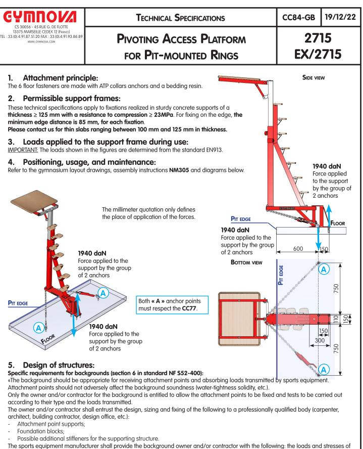
The sports equipment manufacturer shall provide the background owner and/or contractor with the following: the loads and stresses of attachment points taken by the background as regards strength values, types and specifications of the proposed attachments. It is up to the contractor to make the background appropriate for the attachment points in accordance with their locations and the loads provided by the sports equipment manufacturer».
